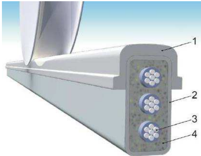
Figure 22: String-Rail Cross-Section (String Transport Unitksy, 2006)
